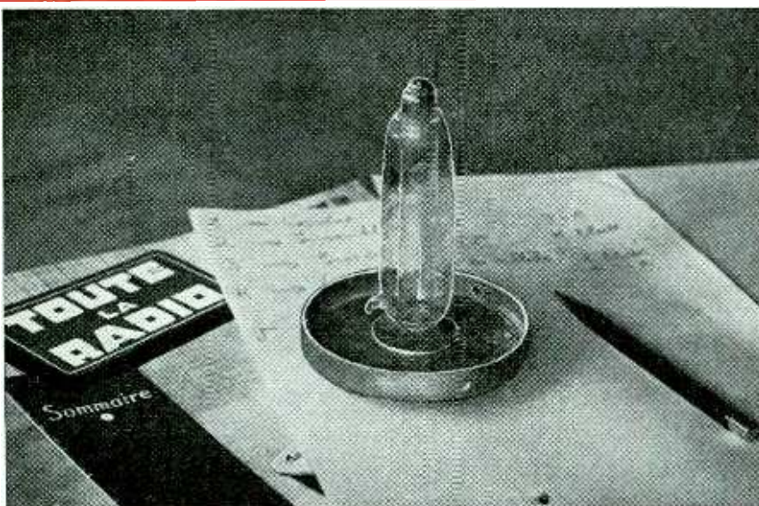
Closeup view of the ionization unit. The opening is down, in the aluminum collar.
