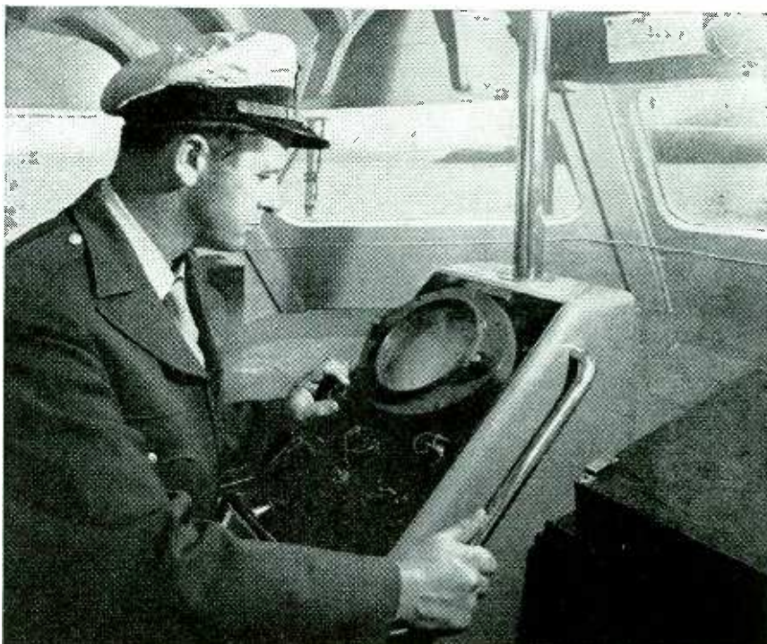
Courtesy General Electric Co. Captain Hooker scans the radar screen aboard the 63-foot patrol boat Bonito. Seagoing game and fish warden uses radar to spot violators off California coast.
