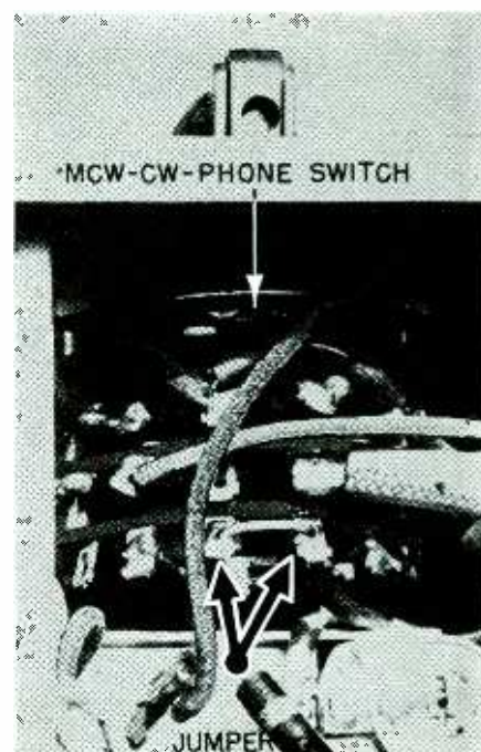
Photo A—Underside, MCW-CW-PHONE switch. Install jumper as shown.
