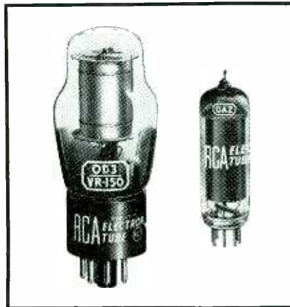
Fig. 1—Cold-cathode gas tube 0D3. The small tube beside it is an 0A2.
